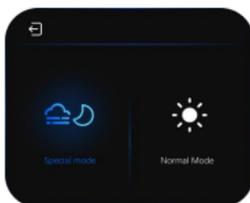
Click a specific mode. After the icon lights up, a pop-up window will appear. Click **Enable** to automatically return to the home screen, indicating a successful setting. If the pop-up displays **This function is already enabled**, it means the current mode is already active, and no further setting is needed. To cancel a specified mode and restore the automatic mode, click **Disable**.
